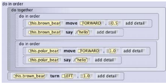
Fig. 1. Parallelism via nested do in order and do together blocks in Alice 3.
